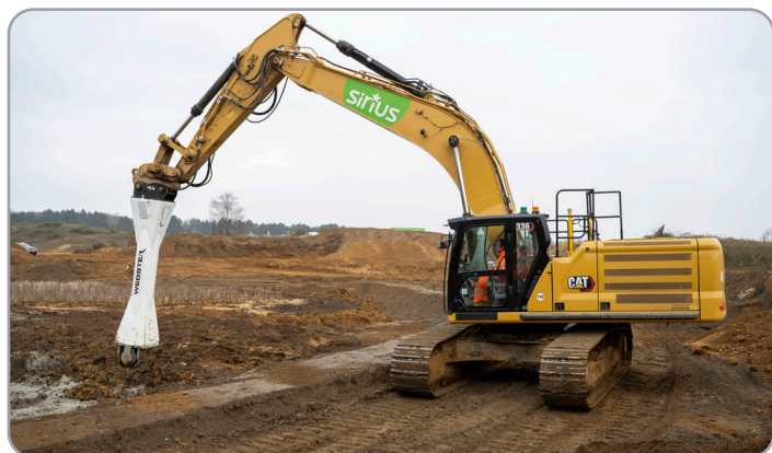
The Sirius G40 mixing wheel with a bespoke, custom made extended boom. The mixing wheel also has a bespoke 'paddle' drum that has flat picks especially for Soil Stabilisation. This is a perfect application for wet mud that needs modifying to create usable soil.
