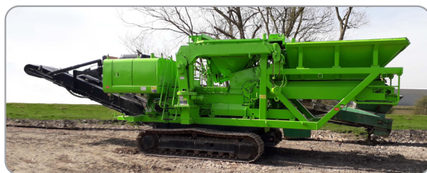
The Sirius STAR Machine (Soil Treatment And Recycling) , turns contaminated soils into reusable material for site.
